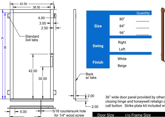
36" wide door panel provided by others. Integrated self closing hinge and honeywell relialign door lock with LED call button. Strike plate kit included with frame.
