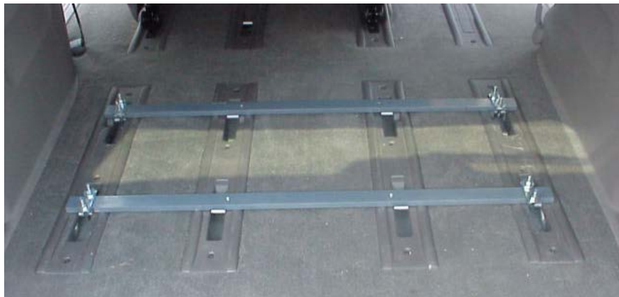
Example: Mounting Bars Installed
